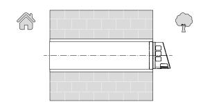
Do not block the air intake grilles or the condensate drain outlet. If necessary, use the supplied mounting wedges (item 3) and sealing foam to ensure that the air duct is fixed in an airtight and immovable manner in the opening.
