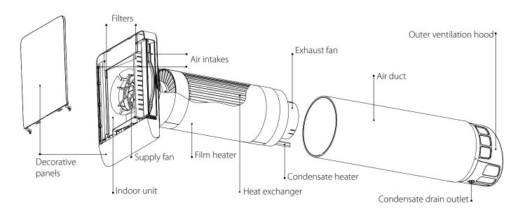
During the operation of the unit, the air flows through the heat exchanger located in the work module. This allows the exhaust air to transfer heat to the cooler supply air, ensuring high quality ventilation.
