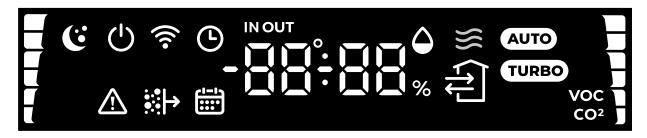
The digital segment of the display shows information such as time, temperature, humidity or all of them in sequence. You can also select the temperature sensor to display (outdoor, supply air, indoor) and select a  $CO_2$  or VOC sensor. The scale on the right shows the fan speed. The scale on the left shows the air quality.
