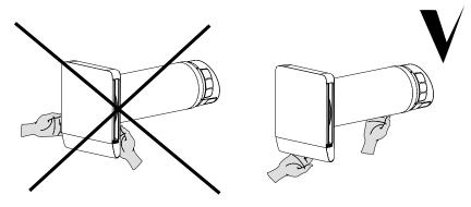
3. Disconnect the air duct and the work module.
