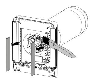
Remove the front panel from the work module. Disconnect the cable and wires.
